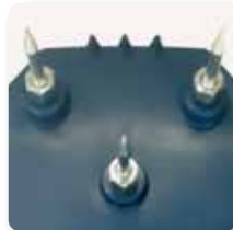
TOE SPIKES PREVENT THE TIP OF THE SHOE FROM CONTACTING THE FLOOR
